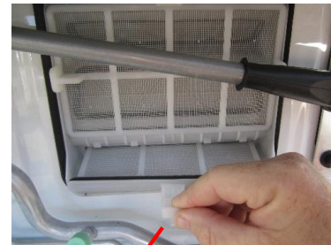
Pull the cabin filter outwards to clean or replace
